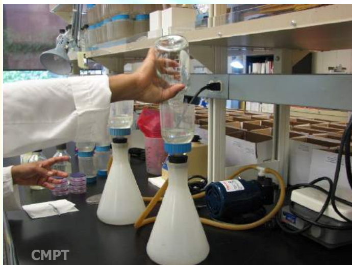
Figure 1. Simple filtration system using a vacuum pump.
