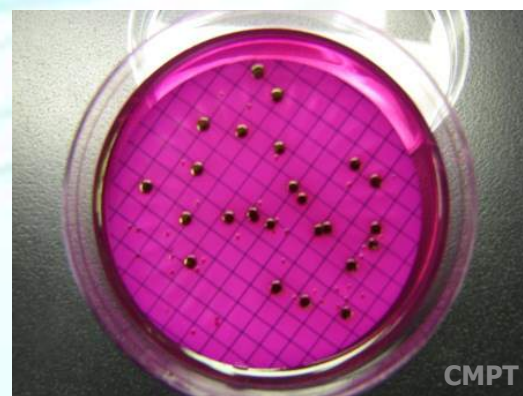
Figure 3. Endo agar plate with two types of colonies: small, pink colonies and larger, with green-metallic sheen colonies (coliforms).
